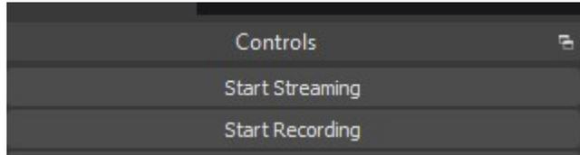
To start the stream you click on the “Start Streaming” button in the Control section of the main OBS screen.
