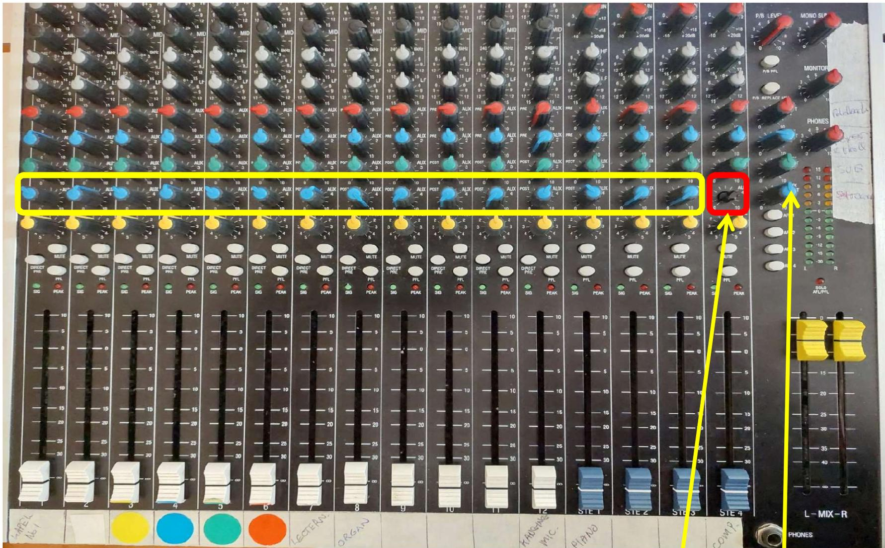
The blue dials indicated within the yellow box are the ones that are used to control the sound level, for the individual sliders, that goes into the OBS software for broadcast for our live stream.
