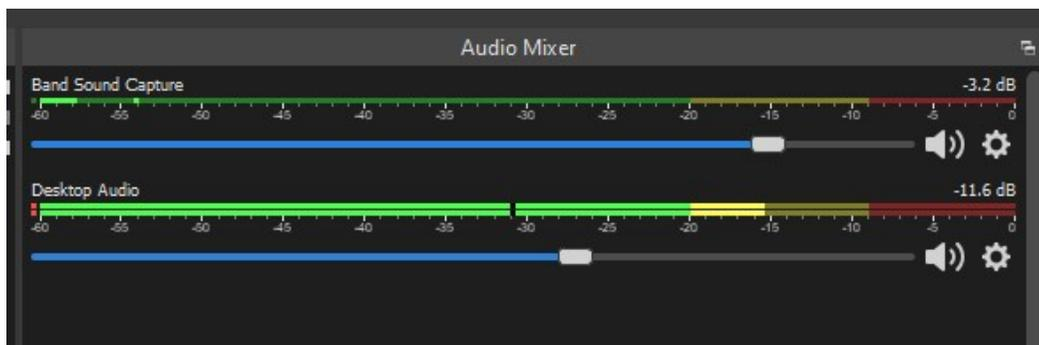
When using the computer for videos or music the sound level does not need to be adjusted as it is set by software. The Blue dial on the desk has been removed to prevent any changes to the input levels. Do not adjust the dial at any time.
