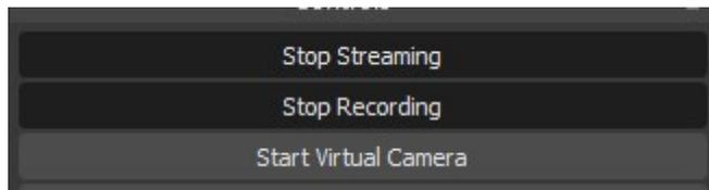
To stop the livestream and recording click the “Stop Streaming” button in the control section of the main OBS screen, this will also end the recording.
